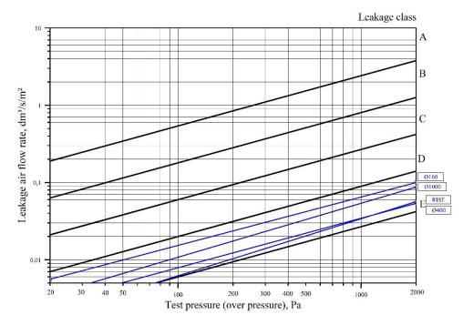
Ventilation duct system VENT meets the certification criteria of the tightness class D both with over- and underpressure. The maximum operating pressure is +2000 Pa/-750 Pa. Components of the certified ventilation duct system VENT are listed in the page 3 of the certificate. Requirements of the certification are listed in the page 4.
